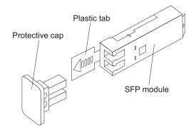
Figure 26. SFP module and protective cap
